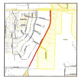
**Description & Scope:** Proposed work includes removal of existing pavement, leveling of gravel base and repavement of new asphalt drive surface. Final site repair and lane striping will complete the project.
